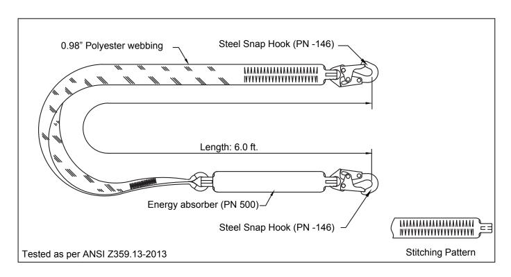
Single leg lanyard incorporated with shock absorber.
